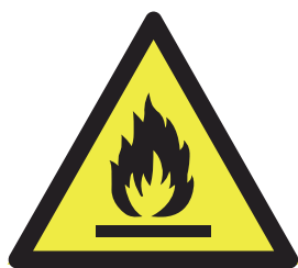
Caution: Risk of fire/ flammable materials
