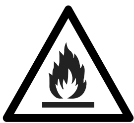
Caution: Risk of fire/ flammable materials
