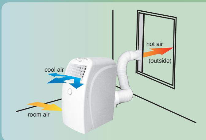
The ability of an air conditioner to cool the air in a room depends on a number of factors including:
